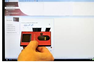
(b) User holding token over flickering pattern (on PC display) to receive a message.
